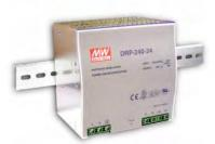
The DIN RP 240 Series are economical industrial DIN rail power supplies with 84% efficiency and built-in protections against short circuits, overloads, over voltage and over temperature. With UL 508 (industrial control equipment) approval and a passive PFC function, DIN RP 240 is reliable in many demanding environments. AC input self switching for use around the world. Wide operating temperature range -10°C ~ +70°C.
