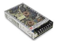
The PS- RSP 100 series is a general purpose, "light industrial level," AC/DC, low profile (1U), single output, enclosed type, switching power supply with Power Factor Correction (PFC).
