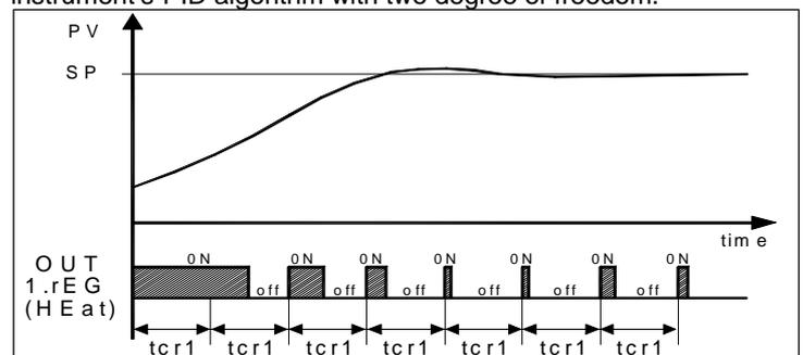
In order to obtain good stability of the process variable, in the event of fast processes, the cycle time "tcr1" has to have a low value with a very frequent intervention of the control output.
