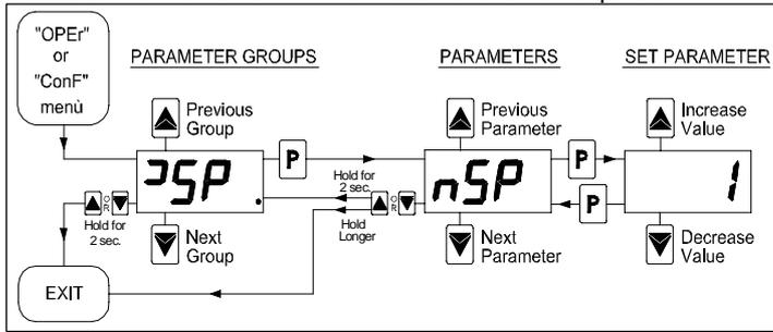
**ATTENTION:** The instrument is programmed in factory with all the parameters, to exception of the Set Point "SP1" (and 2,3,4), programmable in the menu "ConF" to the purpose to prevent wrong accidental programming from non experienced consumers.
