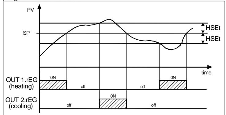
If 2.rEG output is used to control compressor is possible to use the "Compressor Protection" function that has the meaning to avoid compressor "short cycles".
