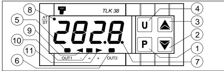
**1 - Key P** : This is used to access the programming parameters and to confirm selection.
