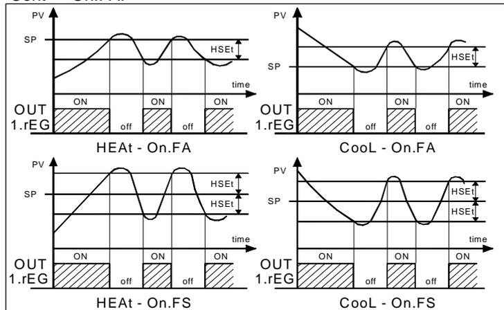
The control works in the following way : in the case of reverse action, or heating ("Func"=HEAt), it deactivates the output, when the process value reaches [SP + HSEt] in case of symmetrical hysteresis, or [SP] in case of asymmetrical hysteresis and is then activated again when the process value goes below value [SP - HSEt].
