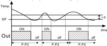
During the output inhibition the led OUT (Cool o Heat) blinking. It is also possible to prevent activation of the output after the instrument is turned on, for the time set in the parameter "P.od". During the power on delay phase, the display shows the indication od, alternating with the normal visualisation.
