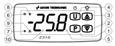
${\bf 1}$  -  ${\bf Key}\ {\bf P}$  : Used for setting the Set point (press and release) and for programming the function parameters (hold pressed for 5 sec.)
