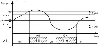
Temperature alarms of maximum and minimum can be disabled by setting the parameters "A.HA" and "A.LA" = oF.
